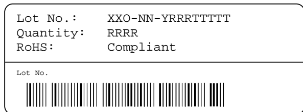
Figure 20: First label on reel: XX = Sensor Type (21 for SHT21), O = Output mode (D = Digital, P = PWM, S = SDM), NN = Chip Version, Y = last digit of year, RRR = number of sensors on reel divided by 10 (200 for 2000 units), TTTTT = Traceability Code.
