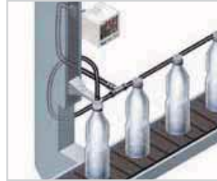
Air-leak test for PET bottles
