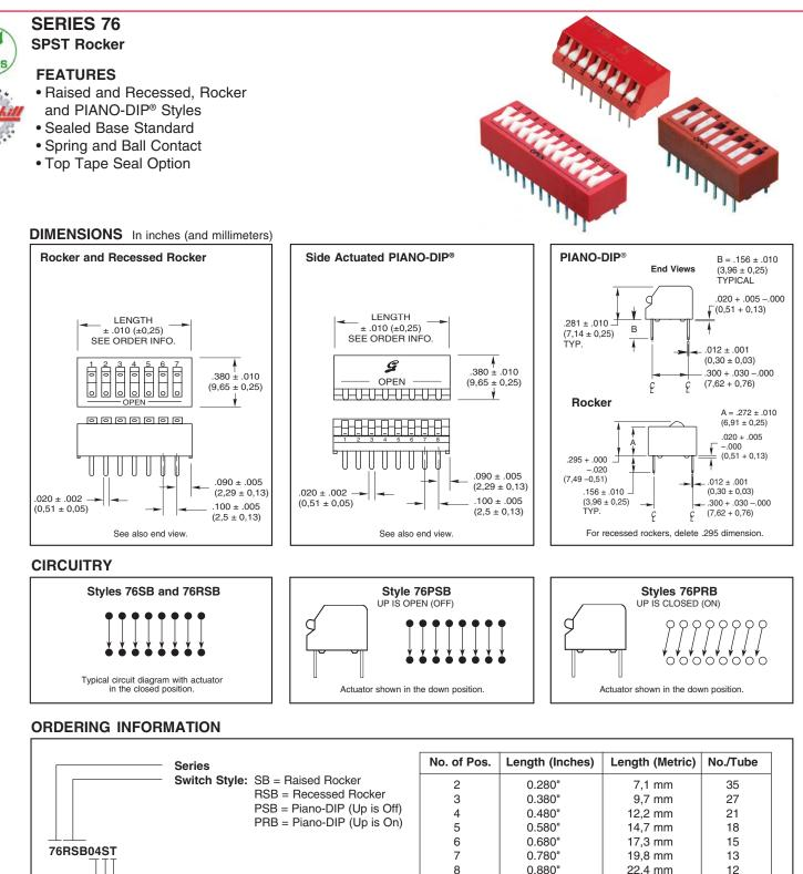
T = RoHS compliant Sealed\*: S = Tape Seal Number of Positions: 02 through 10, 12
