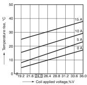
Tested sample: SP4-DC24V Ambient temperature: 27 to 29°C 81 to 84°F
