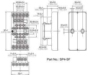
Note: Terminal number marking is on the socket body. Please refer together with the SP relay schematic.
