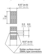
Material: Glass PTFE double-sided through hole PC board R-4737 (Matsushita Electric Works) Board thickness:  $t=0.8\ mm$  .031 inch Copper plating: 18  $\mu m$  Connector (SMA type receptacle) Product name: 01K1808-00 (Waka Manufacturing Co., Ltd.) Value has compensation PC board subtracted only for insertion loss. (Eliminate loss of connector and PC board.)
