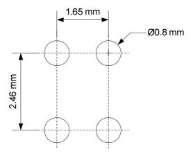
Figure 3 Recommended Customer PCB Land Pattern
