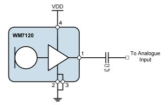
Figure 1 WM7120 Recommended External Components
