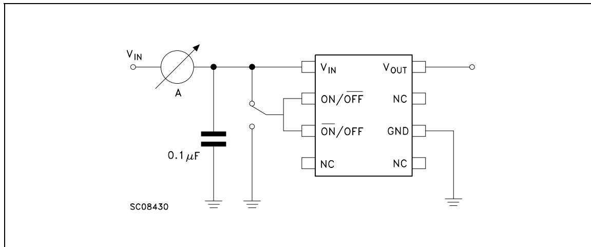
NOTE: The switch emulates the two possibilities to set the regulator in OFF mode.
