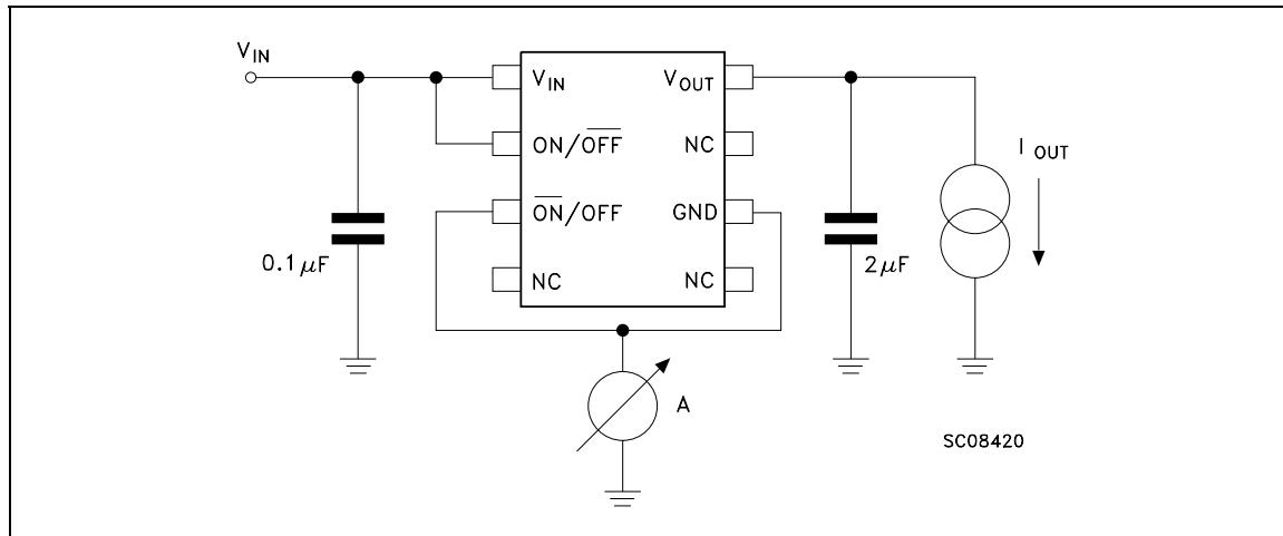
**TEST CIRCUITS:** Supply Current (OFF MODE)
