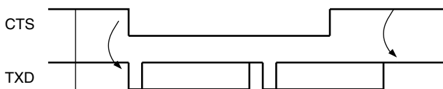
Figure 25-28. Transmitter Behavior when Operating with Hardware Handshaking
