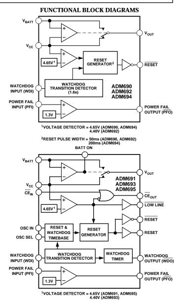
The ADM690–ADM695 family is fabricated using an advanced epitaxial CMOS process combining low power consumption (5 mW), extremely fast Chip Enable gating (5 ns) and high reliability. RESET assertion is guaranteed with  $V_{CC}$  as low as 1 V. In addition, the power switching circuitry is designed for minimal voltage drop thereby permitting increased output current drive of up to 100 mA without the need for an external pass transistor.
