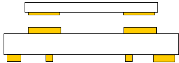
Figure 20. Correct PCB Top Metal Pattern Under Package
