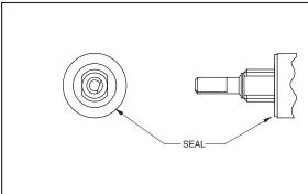
Shaft and panel seal switches are watertight to the panel. They are not totally process sealed like the Style "T". Panel is sealed by a gasket at the base of the bushing. Shaft is sealed by an O-ring inside the bushing. After mounting, seals do not alter switch dimensions. See Style "S" (standard switches) and Style "M" (military switches) in the Choices and Limitations chart.
