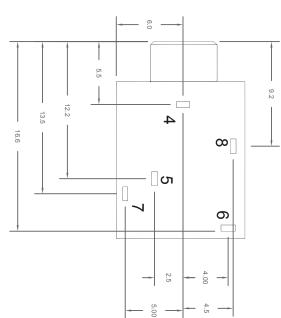
Note: T = Threaded Bushing (M6XP0.5) N = Non Threaded Bushing
