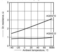
2.-(2) On resistance vs. ambient temperature characteristics
