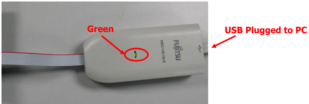
Figure 2.5-1 BGMA Power LED (1)
