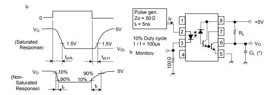
(\*) $C_{\rm L}$  is approximately 15pF which includes probe and stray wiring capacitance.
