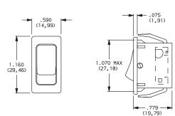
**G2** NEW! ACTUATOR GUARD .050 TYP. (1,27) ſ 1.285 (32.64) SHROUD h / | SHROUD 1.090 (27,69) ŧ R .082 (2,08) TYP. .712 (18, 08)
