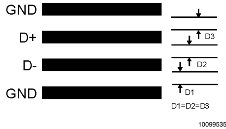
FIGURE 9. Recommended Diode Trace Layout
