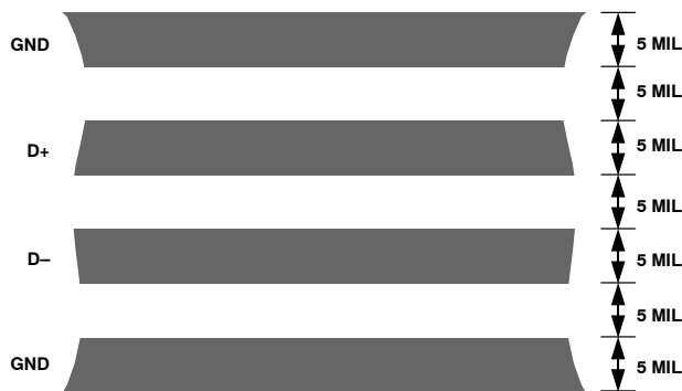
Figure 22. Typical Arrangement of Signal Tracks
