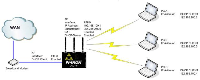
*N-TRON 702-W* configured as a powered Router allows layer 3 routing to set up network segmentation. It supports the Network Address Translation (Masquerading) feature which is widely used by Access Points. NAT will act as the firewall between LAN and WLAN networks. Additional Firewall settings can be configured for Layer 3 packet filtering and access control in Router mode. It can also act as a DHCP server, automating the assigning of IP addresses.
