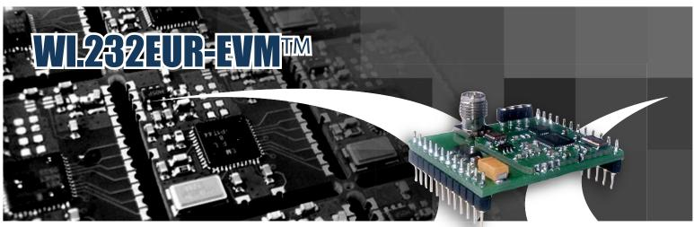
Evaluation Wireless Module 868 MHz, 152.34 kbit/sec.
