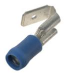
DV14-250P-M Part Number: **RoHS Compliancy** Compliant Status: Piggyback Disconnect, vinyl barrel insulated, 16 – 14 AWG, .250 x .032 tab size. Part Description: Product Type: Disconnects .88 Length (In.): Width (In.): .29 Max. Ins.: .160 Panduit Color Code: Blue Tab Size (In.): .250 x .032 Tool: CT-100A, CT-260, CT-1550, CT-1551, CT-2500 16 - 14 AWG Wire Range: Min. Order UOM: PC Min. Order Qty.: 1000
