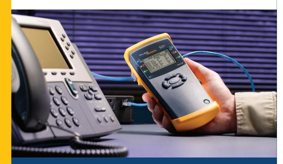
Inline vision between the PC or VoIP phone and network to solve application connectivity problems with the touch of a button
