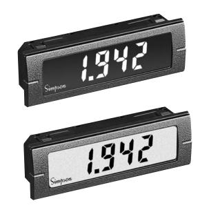
Simpson's Mini DC Current Indicators provide high quality, accuracy, and reliability in a compact 12mm deep case. M135 has a 3-1/2 digit, 0.5" LCD display and is available with a negative image, bright red backlight option. Mini M135s feature user-selectable decimal point and display hold.
