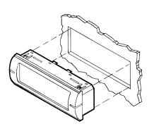
No mounting hardware required, snaps right into panel!
