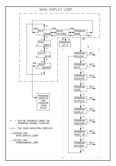
significant digits on the 6-digit Rate display. The desired time units that the rate is to be displayed, can also be programmed as per Second (x1), per Minute (x60), or per Hour (x3600).
