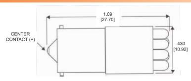
Measurements are typical Dimensions are inches [mm]
