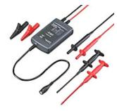
The DP120 differential voltage probe is designed to make measurements on signals with floating reference. The DP120 has two probes with shrouded banana probe tips (one red, one black) and shielded cable for improved noise immunity. Input impedance between each input to shielding BNC is 5 M $\Omega$  in parallel with 6 pF. Input impedance between the inputs is 10  $M\Omega$  with a capacitance of 5 pF.
