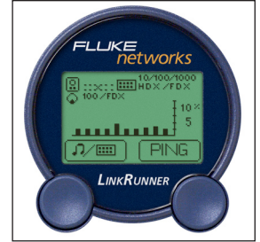
See device capabilities, actual link speed, and utilization levels.
