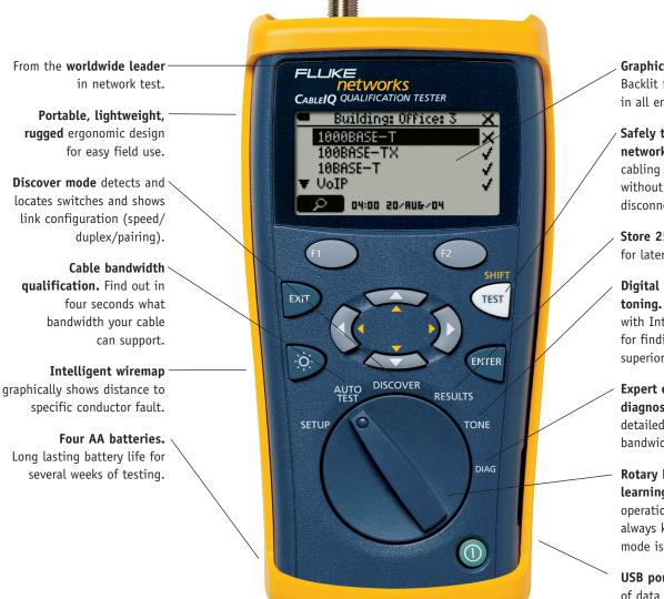
**Graphical display.**Backlit for viewing in all environments.
