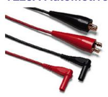
Large jaws, long leads and a piercing probe. Solid, spring-loaded copper clips with a wide 12.7 mm (.50") jaw opening and serrated teeth. Large piercing needle for penetrating larger gauge wires. 1.5 m (60"), silicone-insulated leads, useable from -80 °C to +150 °C (-112 °F to +302 °F). Rated for 30 V, 10 A. One red, one black.
