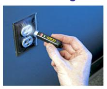
Non-contact AC voltage detector and LED flashlight combined in one convenient, compact design. With exclusive dual-sensitivity. The voltage detector glows blue when it's near AC voltage, and glows red when it's at the source. Detects voltages from 40 V AC to 300 V AC. Voltage detector glows blue 50 Hz - 60 Hz or 2.5 - 38 cm (1 - 5") away from source. Operating temperature 0 °C to 50 °C. Ultra-bright white LED with 100,000 hour bulb life. AAA battery included.
