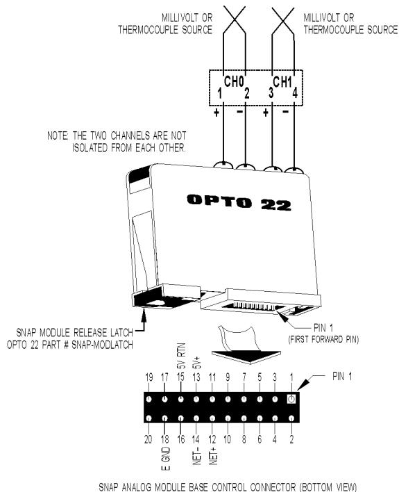
**IMPORTANT:** The mounting rack connector has 24 pins; the module connector has 20 pins. The extra pins on the mounting rack connector prevent misalignment of the module during installation.
