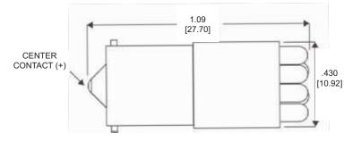
Measurements are typical Dimensions are inches [mm]
