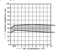
4.-(2) Electrical life (0.5 A 125 V AC resistive load) Tested sample: TQ2SA-12V, 6 pcs
