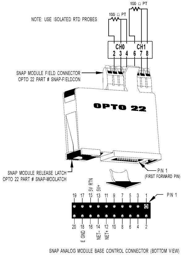
**IMPORTANT:** The mounting rack connector has 24 pins; the module connector has 20 pins. The extra pins on the mounting rack connector prevent misalignment of the module during installation.
