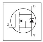
$V_{DSS} = 200V$  $R_{DS(on)} = 0.30\Omega$  $I_D = 9.3A$
