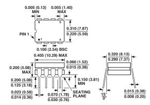
CONTROLLING DIMENSIONS ARE IN INCH; MILLIMETERS DIMENSIONS (IN PARENTHESES) ARE ROUNDED-OFF MILLIMETER EQUIVALENTS FOR REFERENCE ONLY AND ARE NOT APPROPRIATE FOR USE IN DESIGN
