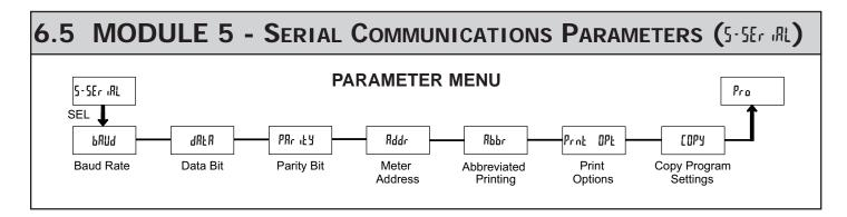
Module 5 is the programming module for the Serial Communications Parameters. These parameters are used to match the serial settings of the CUB5T with those of the host computer or other serial device. The Serial Setup Parameters are only accessible when an optional RS232 or RS485 serial communications module is installed in the meter.
