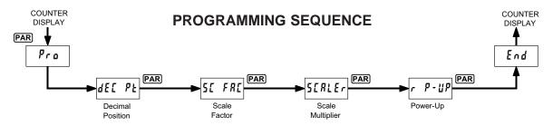
The Totalizer has four programmable parameters which are entered in the sequence shown above, using the front panel push buttons.
