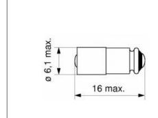
Part Number: 1512135W3D Serial Number: 15121 Based LED type: StarLED Size (inch): T-1 3/4 Size (mm): T6
