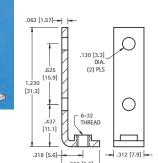
MATERIAL: .062 (1.57) thick Steel, Nickel Plate
