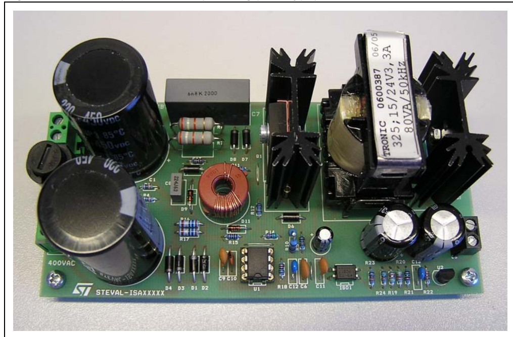
Figure 1. 80 W 3-phase SMPS (working prototype)
