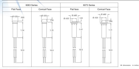
The Chicago Miniature Lamp Glo-Lite Indicator Lights are designed for applications requiring a low cost, line voltage, power-on indicator. These indicator lights utilize a high brightness C2A neon lamp providing good visibility and a long life. These indicator lights are constructed with a one-piece body and lens and are available in two face configurations, flat or conical, with or without a chrome bezel.
