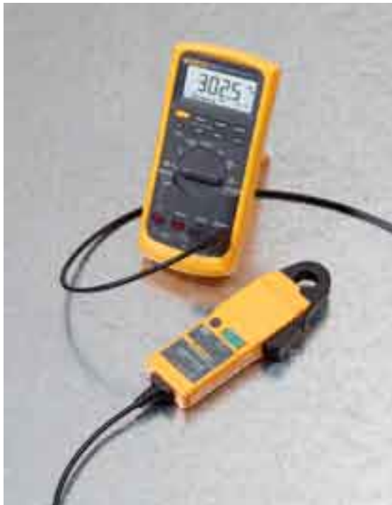
i30 connected to a Fluke 87V Digital Multimeter.
