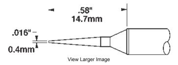
Conical style, 0.4mm, soldering cartridge, 700 series, for use with MX-RM3E Rework Hand-piece or MX-H1-AV Metcal Advanced Hand-piece
