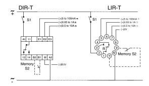
**Note:** Upon energization of the current control IR.T Series Relay, the time delay, which is adjustable from .1 to 10 seconds, inhibits the output relay during start-up periods. The delay time is adjustable via a potentiometer located on the side of the case. Applies to both versions, with and without latching.
