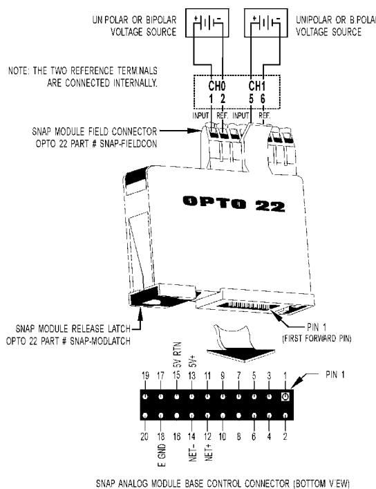
**IMPORTANT:** The mounting rack connector has 24 pins; the module connector has 20 pins. The extra pins on the mounting rack connector prevent misalignment of the module during installation.
