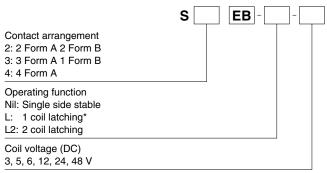
Notes: 1. \*1 coil latching type are manufactured by lot upon receipt of order. 2. UL/CSA approved type is standard.
