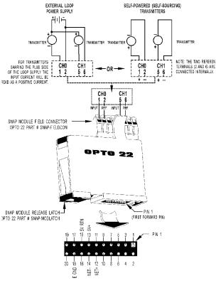
SNAP ANALOG MODULE BASE CONTROL CONNECTOR (BOTTOM V.EW)
