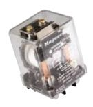
The 785 Magnetic Latching relay, with an Industry Standard square base, operates by using a pulsed input. A permanent magnet maintains the last position until a redirected second pulse moves the contacts back to the original state.
