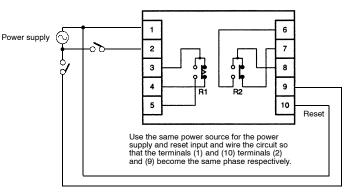
**Note:** The R2 relay can be set to either instantaneous or time-limit contact using the switch located on the bottom of the Timer (H3AM-NS models).
