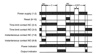
Note: "Rt'" indicates reset input time and "t" indicates set time.
