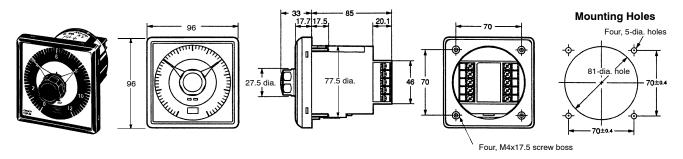
Note: Tightening torque for panel mounting is as follows: 300 m N • m ±50 m N • m (3 kgf • cm ± 0.5 kgf • cm)
