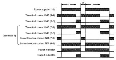
Note: 1. The R2 contacts (7-8 and 6-8) are programmable and can be set to either instantaneous or time-limit contact.
